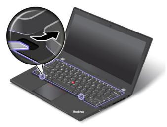
4. Loosen the screws that secure the keyboard with the keyboard multi-tool.
